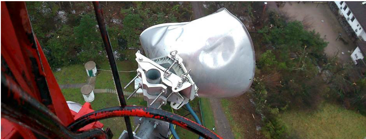
Despite the heavy damage and deformed antenna, the Integra remained operational.
